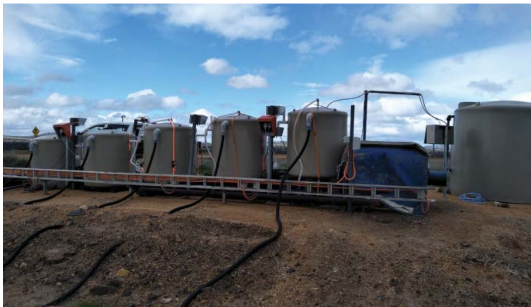
Figure 2. A pilot-scale engineered approach to the biological treatment of \text{SCN}^- -contaminated groundwater at a Victorian gold mine. The bioreactors contain autotrophic and heterotrophic microbial communities capable of degrading \text{SCN}^- , complete nitrification and denitrification. Photo taken by M. Watts.
