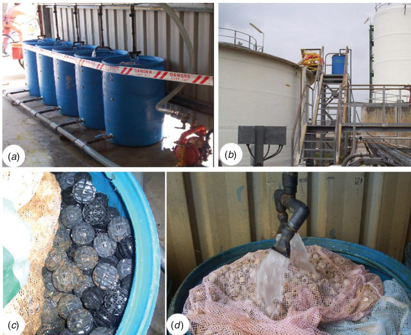
Figure 1. (a) Seed Bioreactor (five drums, 750 L in total), (b) Treatment tank (400 m<sup>3</sup>) (on the left), (c) Bioballs inside each of the drums (placed under the ceramic porous rings), (d) Phenol-contaminated wastewater being added to the netted ceramic porous rings. The phenol contaminated water was added to the Seed bioreactor where the consortium was added and later moved to the treatment tank.
