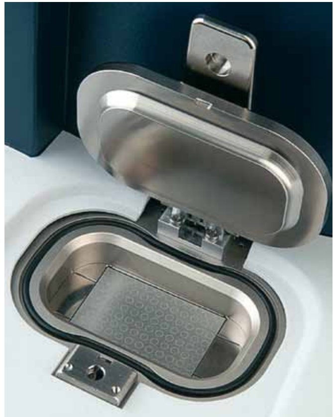
Figure 3. The target plate loaded into the MALDI-TOF.
