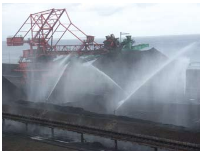
Figure 3. Water used for dust suppression.
