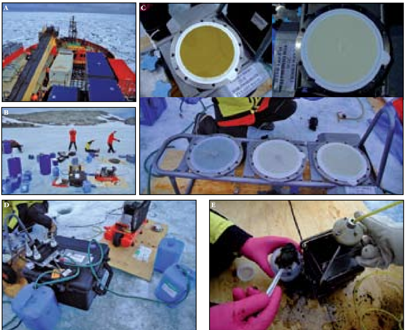
Figure 1. Sampling at Ace Lake for metagenomics and metaproteomics. A) Voyage 2 south on the Aurora Australis. B) The field site on Ace Lake. C) Using equipment from the Sorcerer II GOS, microbial biomass was sampled from various depths throughout Ace Lake and collected sequentially onto 3, 0.8 and 0.1 \mu\text{m} filters. D) The 0.1 \mu\text{m} filtrate was concentrated using a 50kDa tangential flow filter to capture very small cells and viruses. E) Biomass from the bottom of the lake was sampled.
